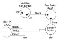
Figure 31 - Blower Wiring Diagram for Thermostat-Controlled Models
